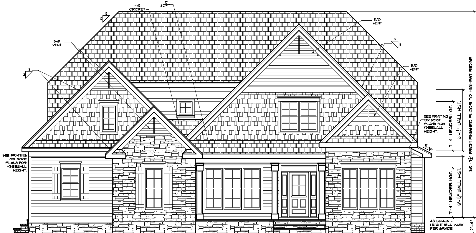
FRONT ELEVATION 1/4"=1'-0" 11x17 PRINTS SCALE: 1/8"=1'-0"
